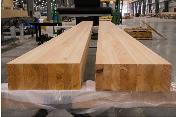
Glulam closeups showing individual wood strips (known as lamella) in cross section [24].
