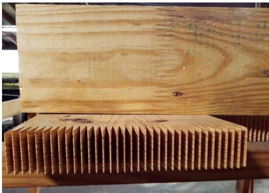
Finger joints (used in both Glulam and CLT). Cutting the ends of beam segments this way maximizes the contact area between them, allowing glue to hold together as much material as possible, maximizing strength [25].
